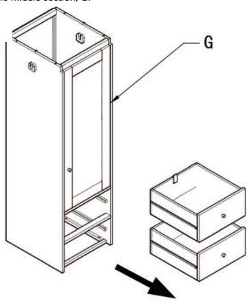
4. Using 6 of the allen key bolts  $\,L\,$  attach the middle section to the base of the wardrobe  $\,(E)\,$  as shown.
