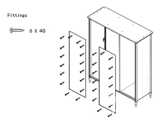
7. Using the 2x 30mm screws, N, attach the top panel to the sides through the pre drilled holes inside the wardrobe. Attach the bottom of the middle section to the bottom of the wardrobe as shown below. Then attach the L/R doors onto their hinges. Attach the door panels onto the side panels as shown below.
